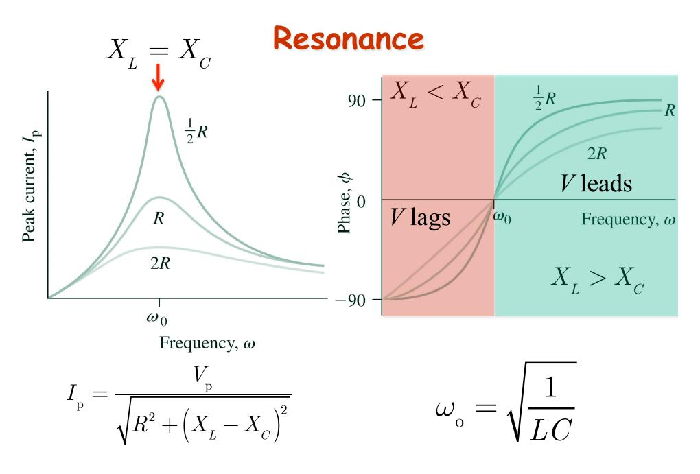
At resonance, Z = R, and  $\phi = 0$  (just like a DC circuit)
